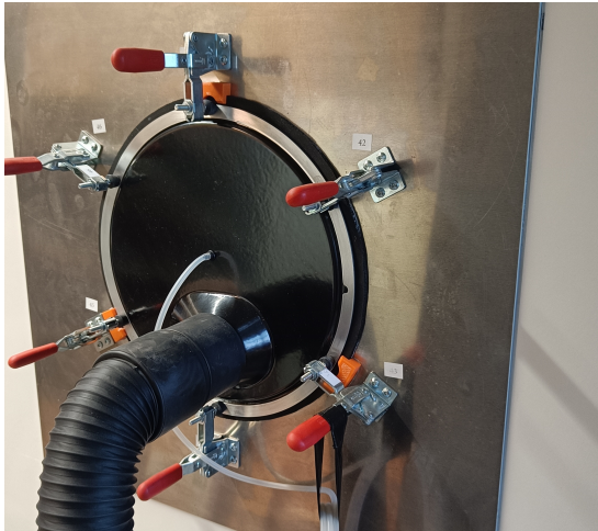
(a) Connection adapter of the Minneapolis DuctBlaster to the ATLAS
