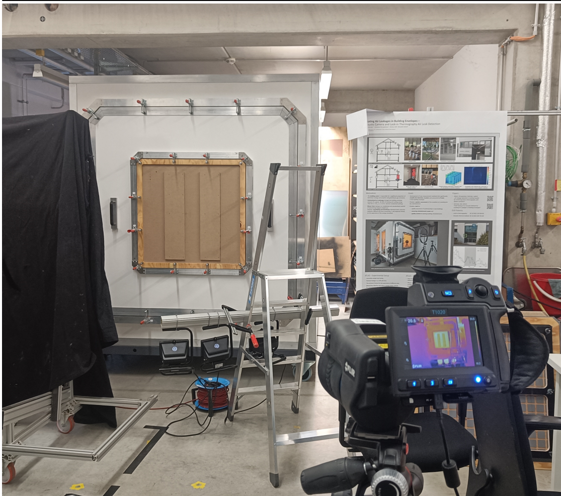
Figure 13 Measurement setup. The ATLAS Test bench with an a test specimen, halogen lamps to simulate sunlight and the FLIR T1020 infrared camera. Researchers can hide behind the curtain to mitigate unwanted disturbances.
