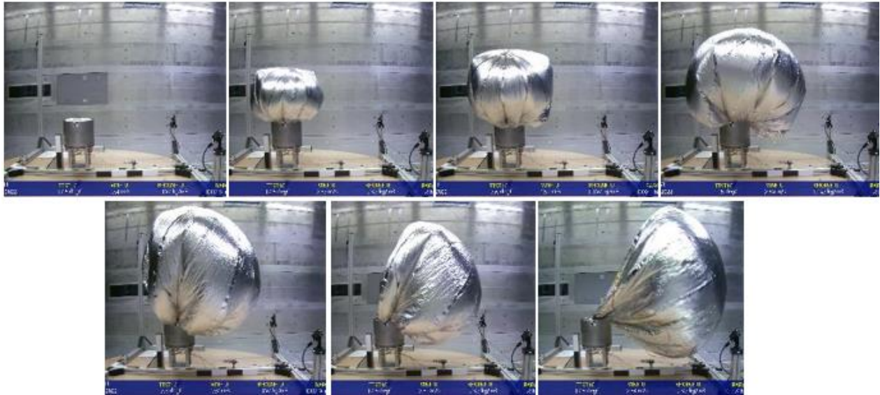
Fig 6 Inflation image sequence obtained during wind tunnel tests. Lower right image: fully blown down to \sim 65^\circ at 2.5 m/s ( \sim 4.0 m/s on Mars)
