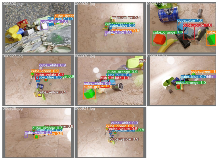
Figure 7.7.: Example of YOLOv7 validation output on a test data batch.
