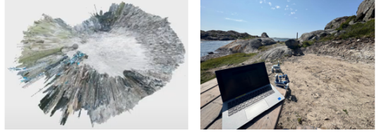
Fig. 8. 3D map of a sand pit of approximately 23 m 2 , generated through Breadth-First Search autonomous exploration, validating the correct implementation of RAFCON state machines, perception capabilities, and autonomous task execution.
