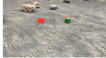
Fig. 6. Trained YOLOv7 object detector output, running on the rover’s on-board computer, in the PEL laboratory, on colored cubes near rocks.
