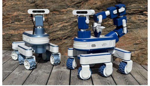
Fig. 1. Picture of the Lunar Rover Mini 1, on the right with the robotic arm, and the Lunar Rover Mini 2, on the left.
