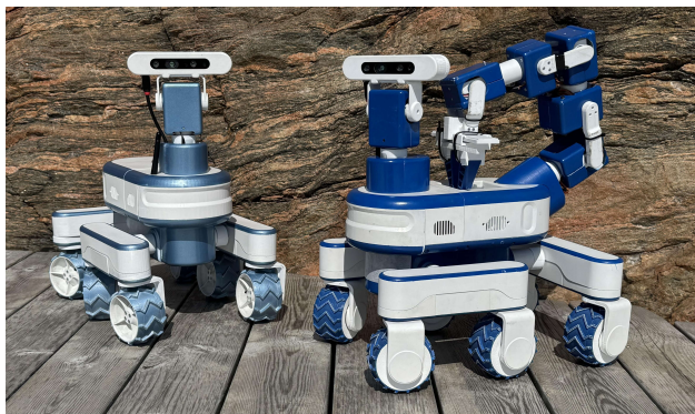
Figure 1.1.: Picture of the Lunar Rover Mini 1, on the right with the robotic arm, and the Lunar Rover Mini 2, on the left.
