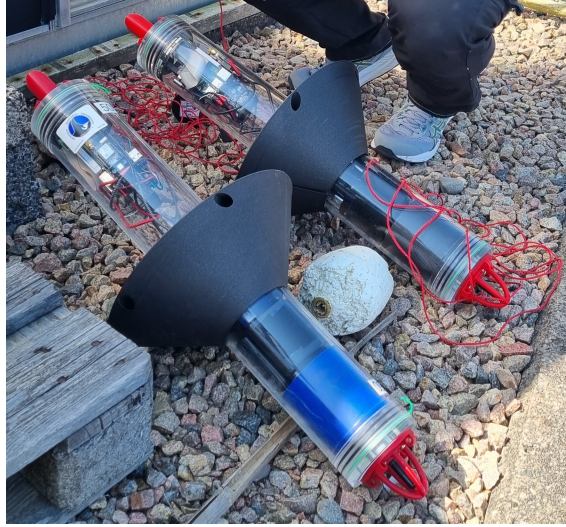
Figure 6.1.: Tubes with hydrophones and GPS receivers that served as ASVs.
