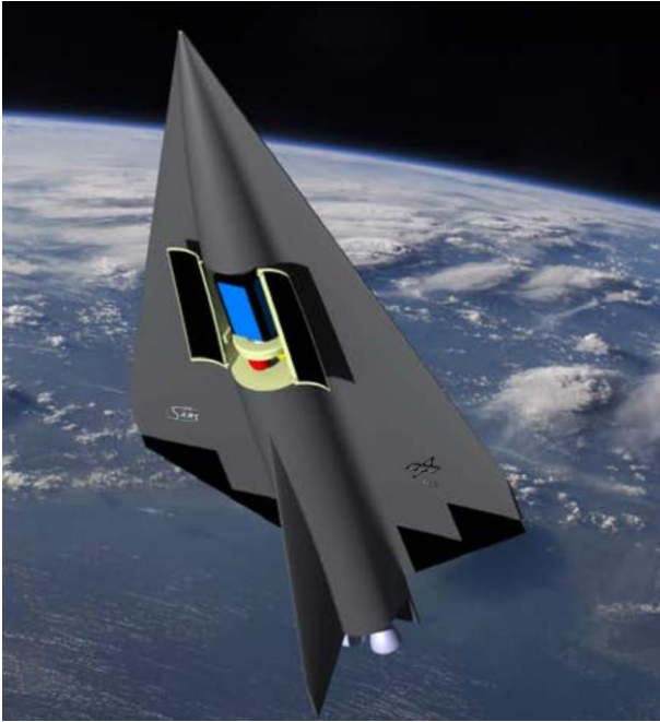
Figure 8: SpaceLiner 7 orbital stage (SLO) in rendering with open cargo bay
