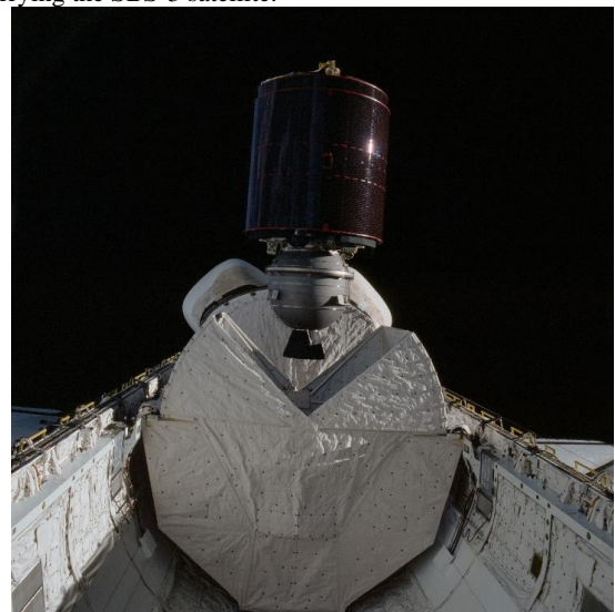
Figure 2: PAM-D with SBS-3 satellite being deployed from Space Shuttle Columbia during STS-5 mission, [11]
