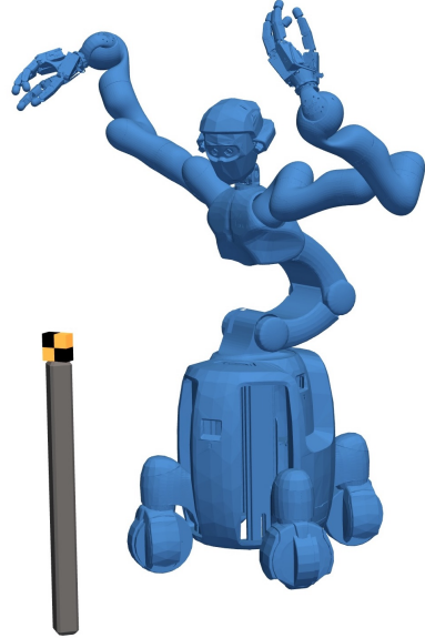
Fig. 1. DLR's Agile Justin [2] collecting measurements using its head-mounted RGB camera for the calibration of its elastic forward kinematics as well as the camera's intrinsic and extrinsic parameters. Only simple markers on both hands as well as the depicted marker mounted on a pole are used. As described in Section V, we select filtered random configurations to identify the robot in its whole work space.
