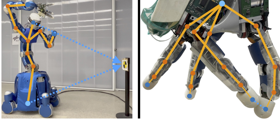
Figure 2.1: Calibration of two complex mechatronical systems; left : vision-based calibration of the humanoid Agile Justin [Bäu+14] with internal RGB camera. right : contact-based calibration of the DLR-Hand II [J B01].
