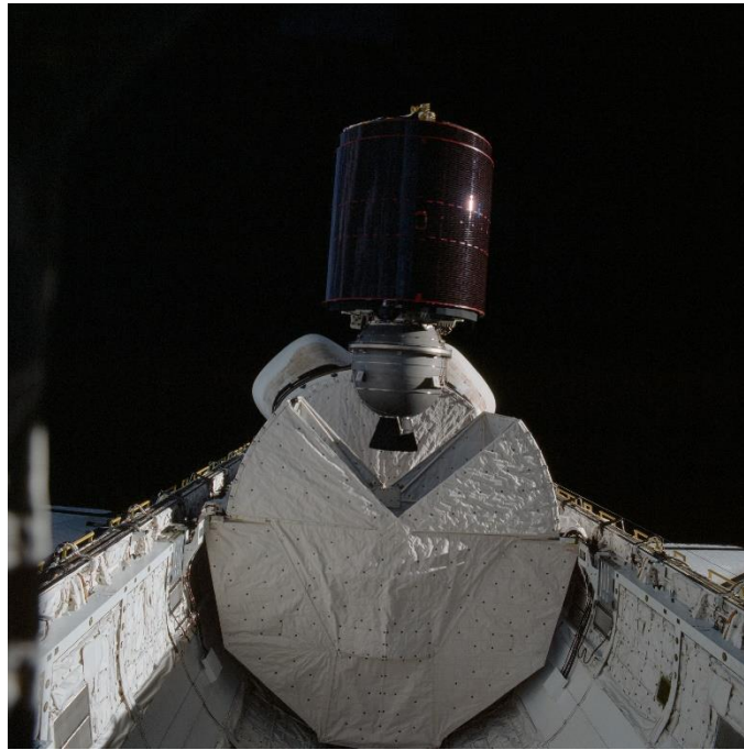
Figure 2: PAM-D with SBS-3 satellite being deployed from Space Shuttle Columbia during STS-5 mission, [8]
