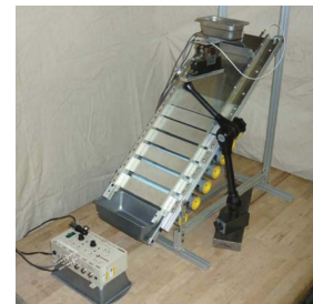
(e) LSPS slotted ramp separator [12].
