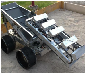
(c) Bucket-ladder excavator of 2013 Lunabotics competition. (Image credit: Lichtenheld et al. [8])
