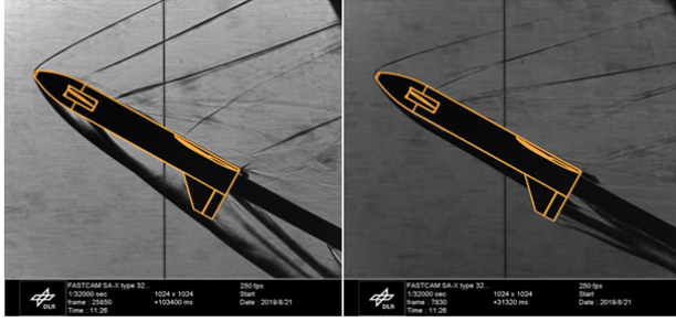
Fig. 6: Schlieren images of the ReFEx model during a Mach 2.5 (left) and Mach 4.5 (right) run; canard angle -5^\circ , angle of attack 28^\circ .
