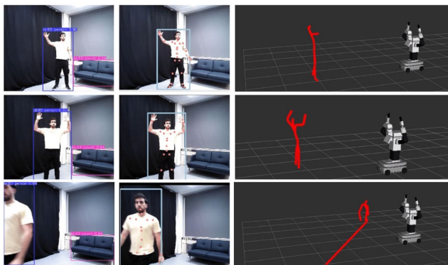
Fig. 9 End-to-end pipeline of our real-world robot control for social human-robot interactions. Here we do not showcase any robot behavior, but the overall human capture system. First, we use YOLOv9 [69] and HybridIK [70] for human detection and pose estimation. Then, we transform all the coordinates to the robot’s coordinate frame and generate the robot behavior accordingly
