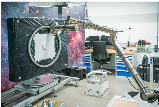
Figure 12. EROSS: CAESAR arm performing the capture of an unprepared client. Credit: DLR.
