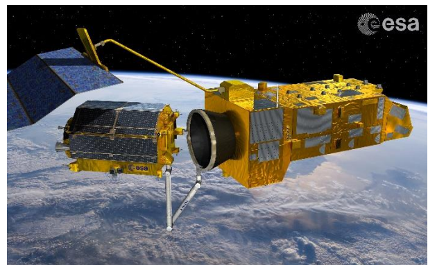
Figure 8. e.Deorbit's robotic arm. Credit: ESA.
