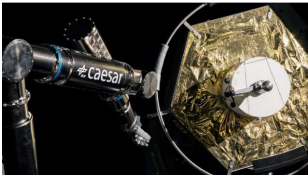
Figure 6. CAESAR robot arm. Credit: DLR (CC BY-NC-ND 3.0).
