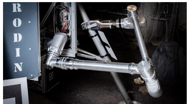
Figure 7 Stable: DLR Space Arm Technology mounted on a lander to demonstrate autonomous work. Credit: DLR (CC BY-NC-ND 3.0).
