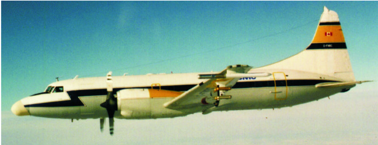
Figure 4-4: Image of Canadian NRC Convair-580 Aircraft Equipped with Meteorological Probes [9].
