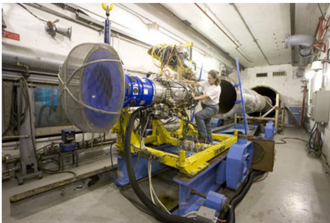
Figure 4-21: NRC-TC5 Turbojet on Thrust Stand.
