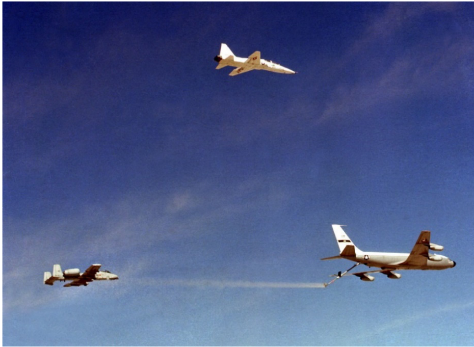
Figure 4-34: Example of Spray Tanker Test with Three Different Aircraft Involved [66].
