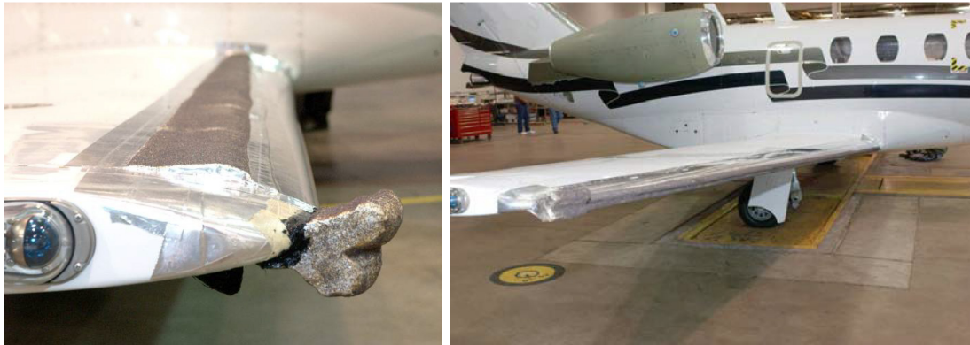
Figure 4-7: Flight Test with Simulated Ice Shaper: (Left) Runback Shape and (Right) Wing Ice Protection System Failure Case [25].
