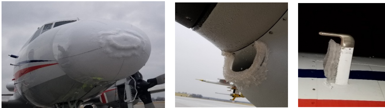
Figure 1-1: Ice Accretion on Different Part of an Airplane; Left: Nose; Mid: Engine Inlet; Right: Sensor Probe. Courtesy of NRC Canada, Flight Research Laboratory.
