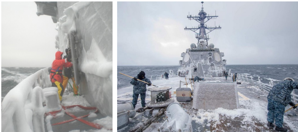
Figure 1-2: Typical Ice Accretion on Sea Vehicles; Left: HMNZS WELLINGTON in the Ross Sea (Feb/Mar 2011), Courtesy of Chris Howard, Chief Naval Architect, RNZN; Right: Sailors Battle Ice on USS McCampbell ( https://navaltoday.com/2017/02/08/uss-mccampbell-sailors-battle-ice-ahead-of-japan-port-call/ ).
