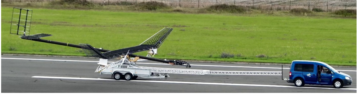
Figure 7: HAP-Alpha on launch vehicle during taxi test
