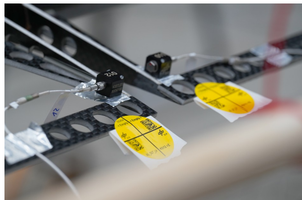
Figure 2: The aircraft during ground vibration test (top), excited by elector-magnetic shakers (left), vibrations of the primary structure measured by accelerometers (right)
