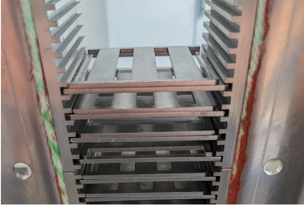
Fig. 25 Heat exchanger channel while assembling the “w10 h02 n3 z10” packing structure.
