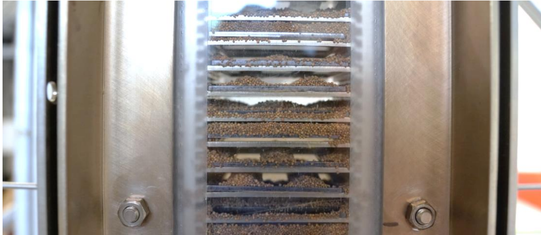
Fig. 26 View in the “w14 h02 n2 z10”-packing structure with static particles during cold testing.
