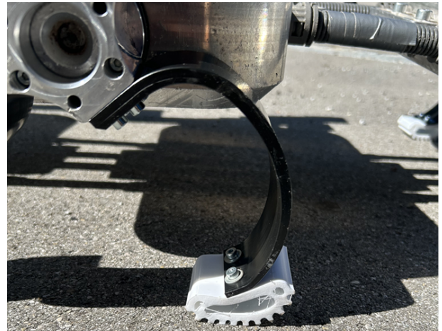
(a) Foot connection on previous spoke design under load
