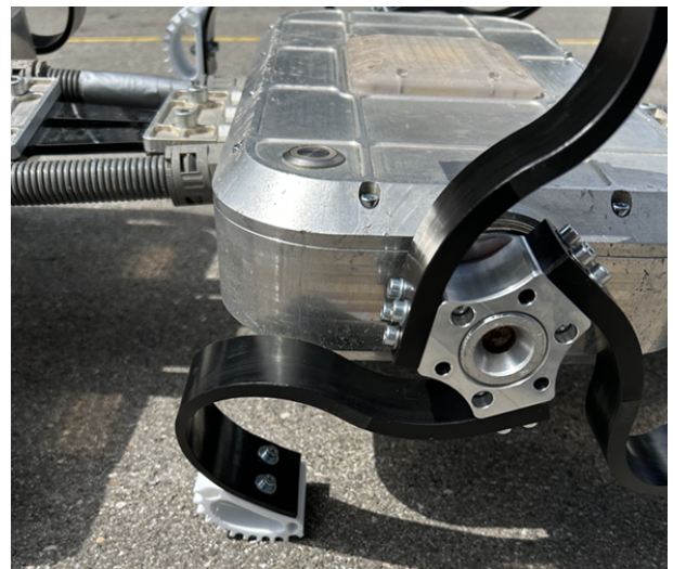
(b) Foot connection on revised spoke design under load
