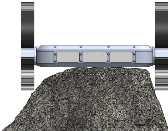
(a) Previous spoke design interacting with a large stone; chassis contact occurring regardless of wheel orientation
