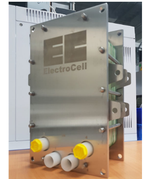
Cell and Stack for SDE in the experimental setup at DLR
