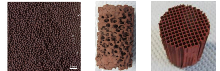
Metal oxide structures 3, 4, 5 employed for catalytic Sulphuric Acid Splitting in DLR
