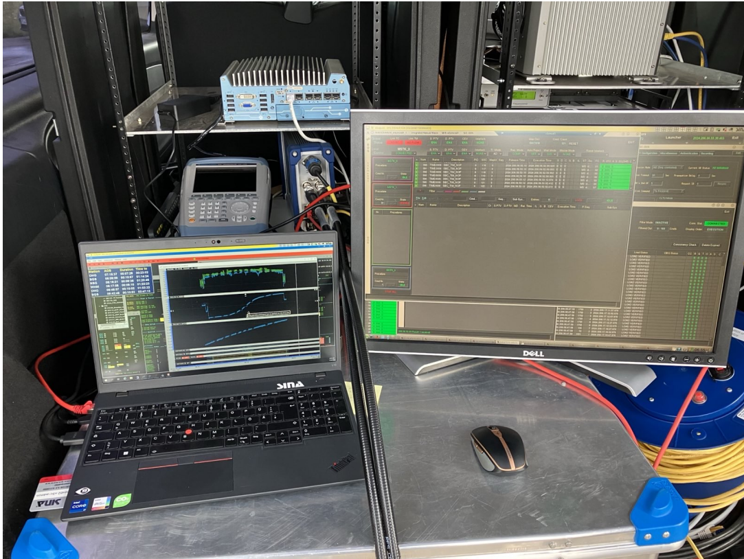
Fig. 8 Photo of V3C in trunk compartment of van during GEO relay demonstrations. The laptop shows visualizations of various satellite telemetry parameters, the connected monitor shows successfully uplinked telecommands. Some communication equipment for the relay link can be seen in the background.
