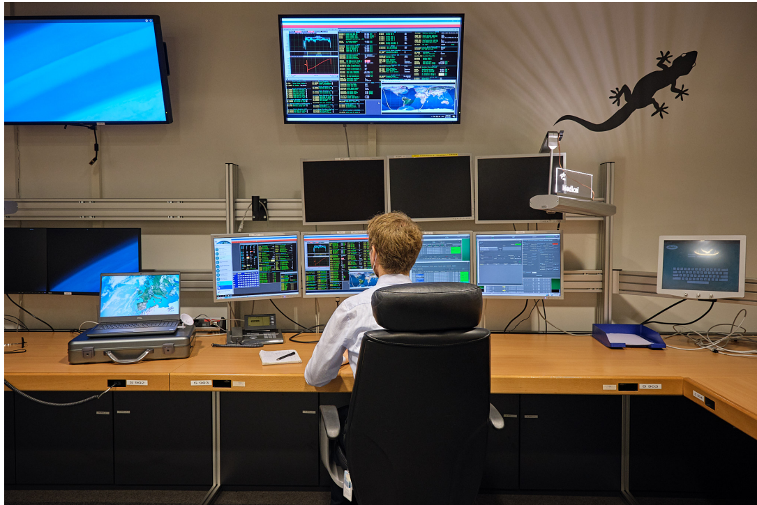
Fig. 2 Setup of V3C (laptop on the left) in one of GSOC's control rooms during the first demonstration campaign. V3C is accessed from the console via remote desktop connections, no other infrastructure except connection to the ground station is used.
