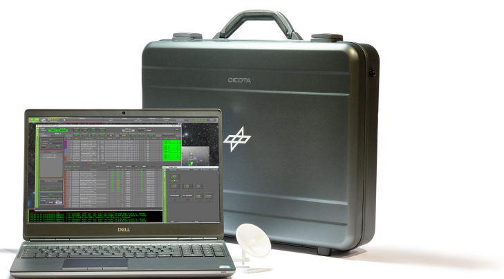
Fig. 1 V3C as a mobile solution for satellite operations independent of ground infrastructure except for some means to establish a communication link with the spacecraft (symbolized by the 3d-printed antenna), runnable on mobile COTS hardware.
