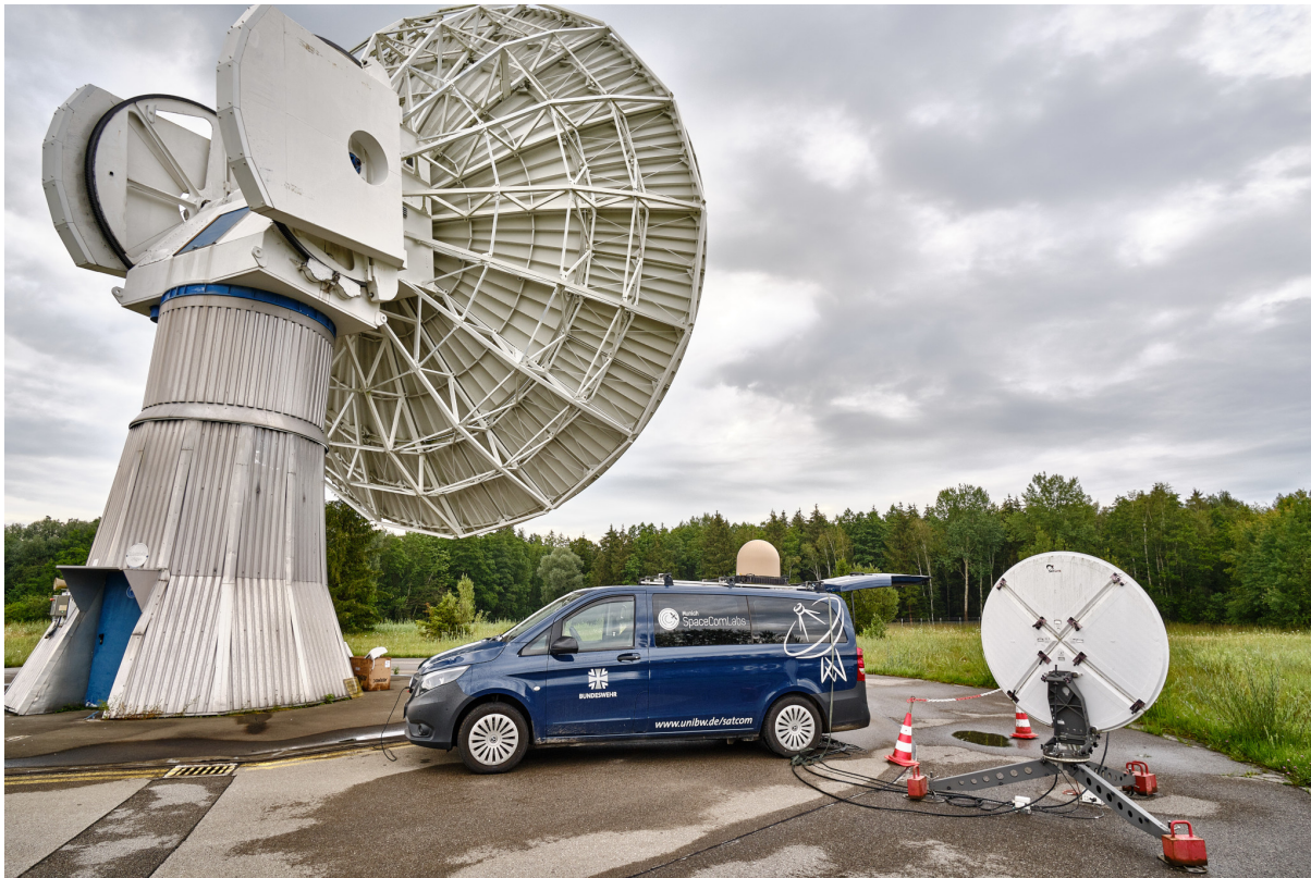
Fig. 7 Photo of communication van (center) with SOTM antenna (on the van’s roof top), S-band tracking antenna (left) and VSAT antenna (right) during GEO relay demonstrations.
