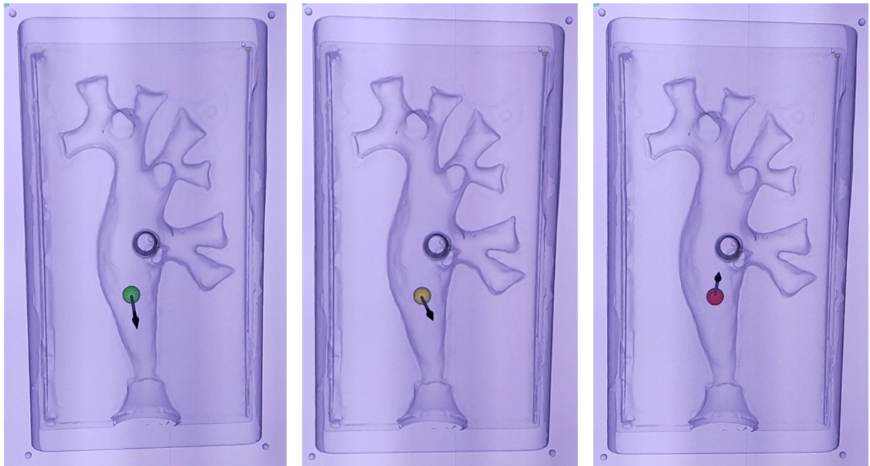
Fig. 3.25: RViz: the ball represents the endoscope tip, and the color changes according to the distance from the walls of the kidney - green : safe distance, yellow : borderline-safe distance, red : threshold distance, about to collide with the wall
