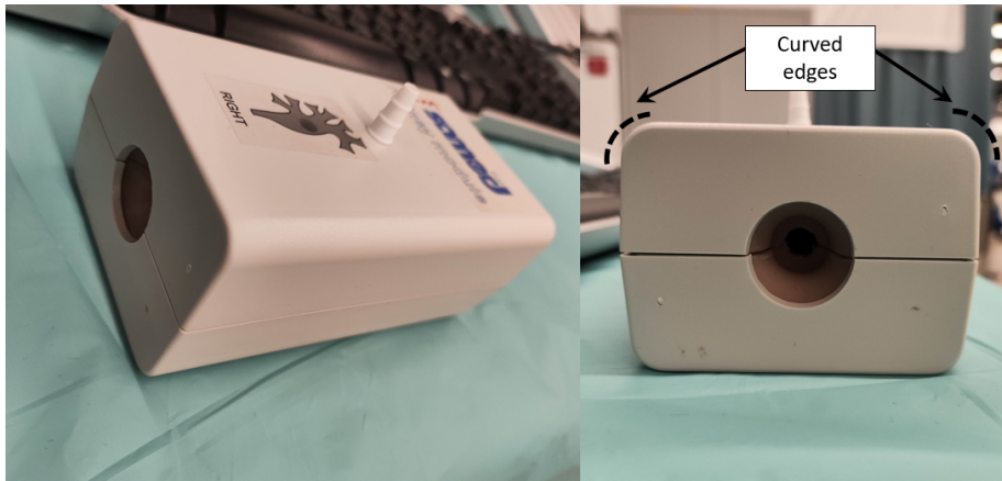
Fig. 3.14: Curved edges of the kidney phantom box
