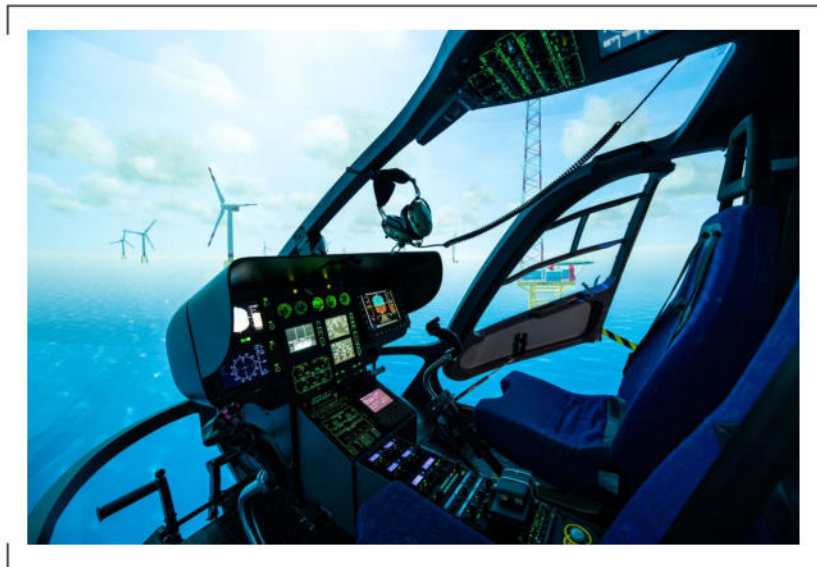
Figure 4.5.: AVES ACT/FHS Cockpit with Dome Projection of a Maritime Offshore Wind Farm. 2
