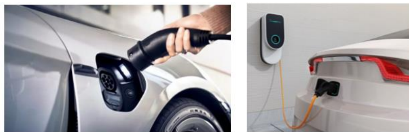
Figure 26: Electrical Interface/Coupling with a Type 2 charging connector; Installation space of approx. 80 mm x 80 mm x 75-90 mm (WxHxD) (Golem.de, 2024; Schwäbisch Hall AG, 2024)
