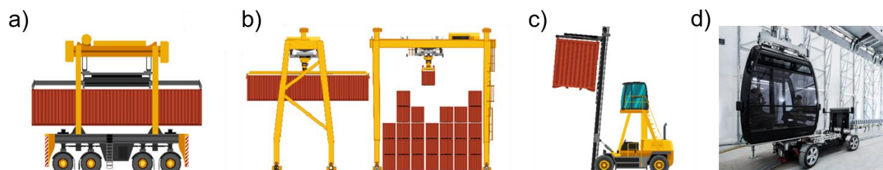
Figure 22: Roof handling devices, used in industry. a) Straddle/Shuttle Carrier for shipping containers. b) Stacking/Gantry crane. c) Top pick crane truck. d) ConnX prototype by Leitner AG (J&S Maritime Ltd, 2024; Leitner AG, 2024)
