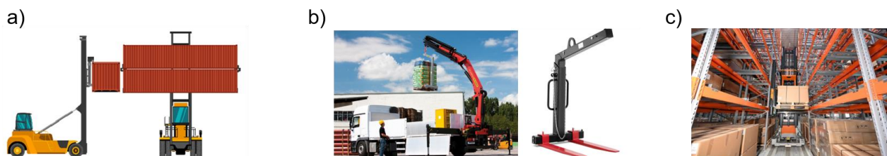
Figure 21: Forklift handling devices, used in industry. a) Forklift trucks and empty handlers for shipping containers. b) Mobile forklift adapter for cranes. c) Automated high-bay warehouse mover (J&S Maritime Ltd, 2024; Palfinger AG, 2024; CDN, 2024; Pressebox, 2024)
