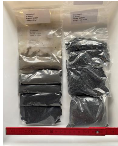
Figure 2 – sorted sample from the surface of the patch in figure 1, based on the grain size. Similar work has been done for the samples taken from subsurface.
