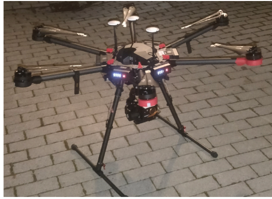
Fig. 6. The UAV system applied for the pilot application, with the thermal camera attached via gimbal.
