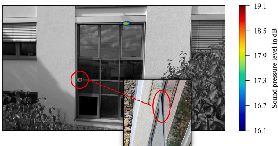
Fig. 8. Detected leakages at a large window front. The frequency range from 5.4 kHz to 6.0 kHz was selected to superimpose the sound pressure level on the photograph.
