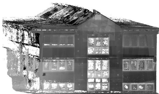
Fig. 12. Point cloud textured with infrared imagery.
