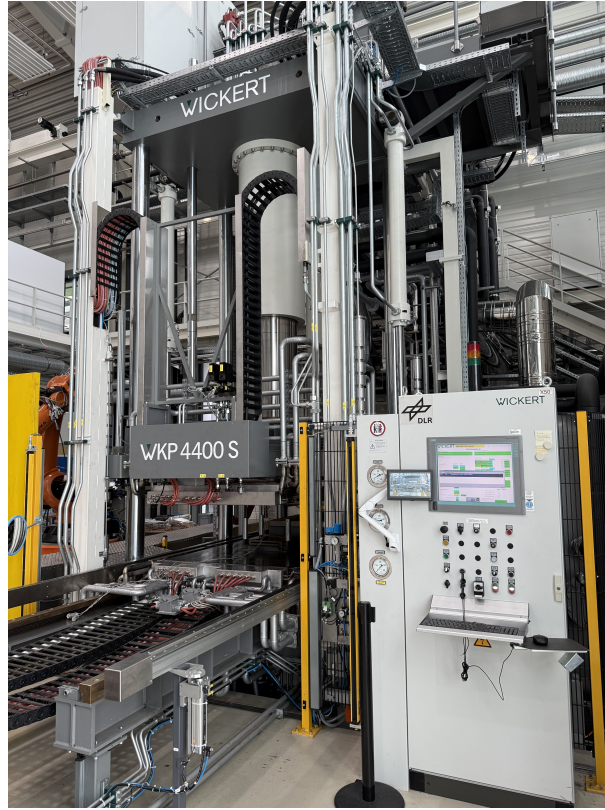
Figure 3.1: Wickert WKP 4400S industrial hydraulic press.
