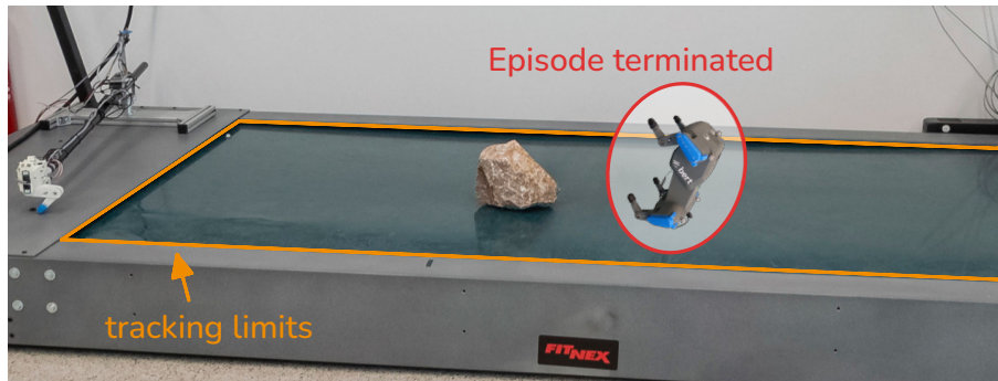
(b) The episode terminates because the robot falls (early stopping)
