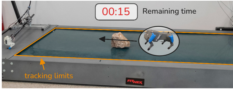
(a) Experimental setup of a quadruped robot on a treadmill.
