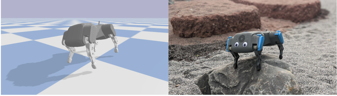
Figure 6.5: Robotic quadruped with elastic actuators in simulation (left) and real hardware (right)
