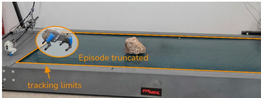
(d) The episode ends because the robot reached the limits of the tracking device (truncation).
