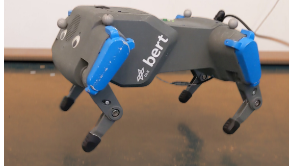
Figure 2.11: Compliantly actuated DLR quadruped bert jumping in place.
