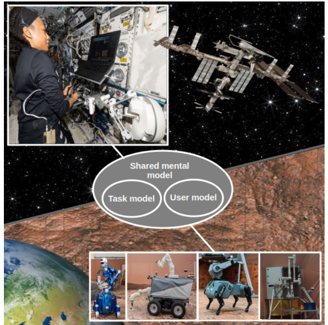
Fig. 4. A SMM supports the astronaut during teleoperation of robotic assets. The top picture shows NASA astronaut Jeanette Epps on-board the ISS during a Surface Avatar orbit-to-surface telerobotic experiment session in July 2024 and the bottom right shows the robotic team which she commanded, consisting of Rollin’ Justin, the Interact rover, the quadruped Bert and the lander arm. Creating an SMM between astronaut and robot includes estimating the task goal, as part of the task model, and including individual user preferences, as represented in the user model.
