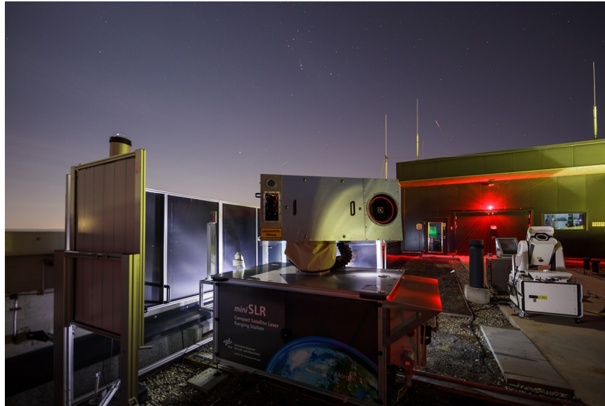
Figure 2.11.: The miniSLR ® system at the DLR site in Stuttgart. From this station on the roof, high-precision distance measurements to satellites are performed using laser pulses (Photo: Paul Wagner / DLR).
