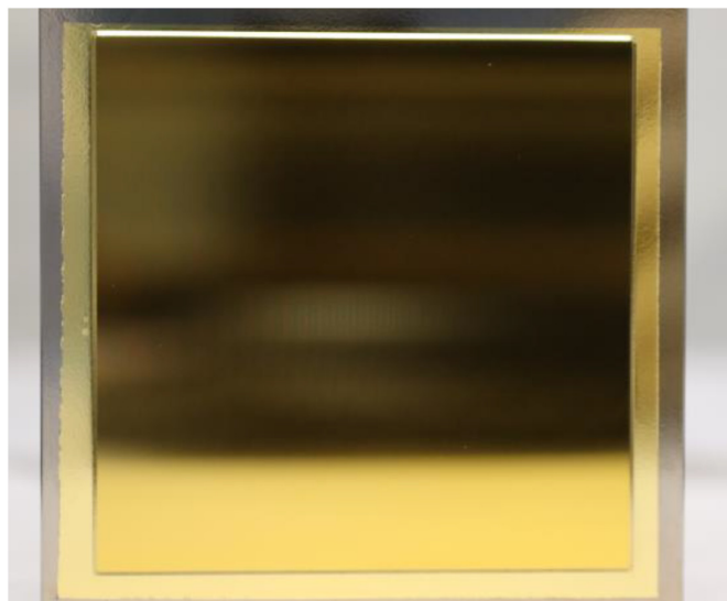
Fig. 10 Grating after coating.
