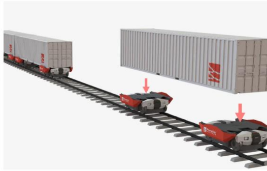
Figure 10 Parallel systems - Self-propelled traction units [23]
