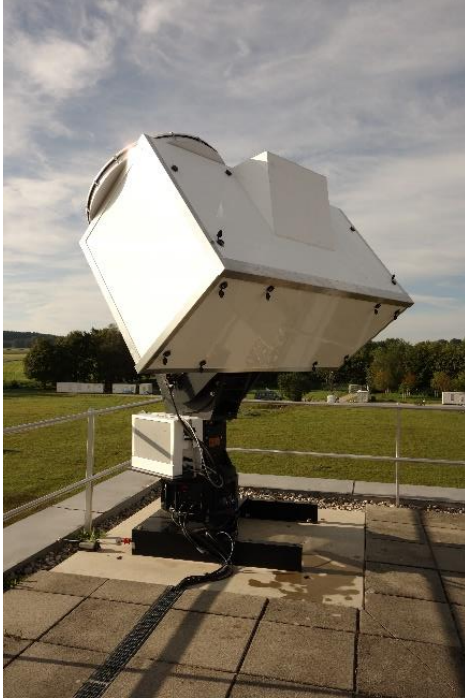
Figure 3: Image of the DLR's novel /L-/X- dual-band transponder prototype.
