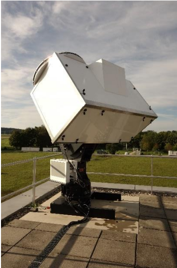
Figure 1: DLR's novel dual L- and X-band calibration PARC designed for ROSE-L.
