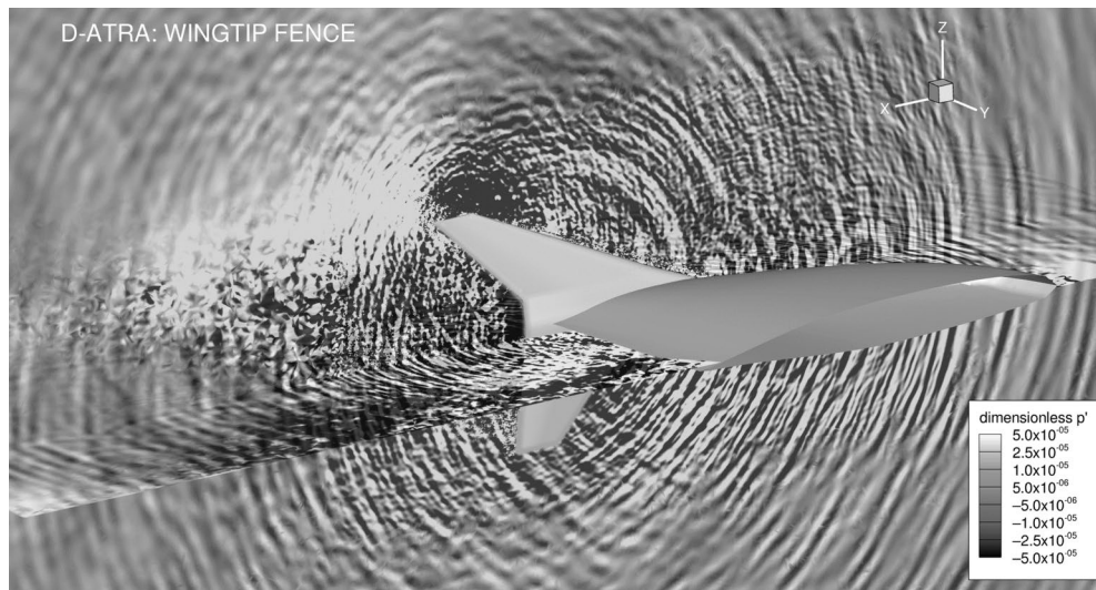
Fig. 15 D-ATRA wingtip fence contour slices, showing instantaneous pressure fluctuations
