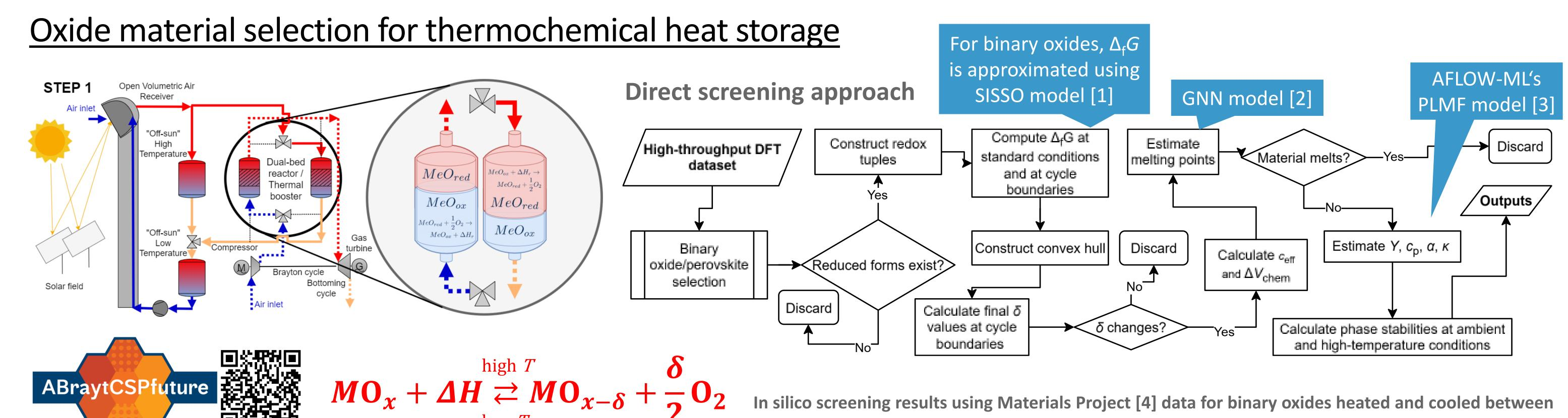
Goal: Identify metal oxide materials which can store maximum amount of sensible heat + chemical heat via a reversible redox reaction in an oxygen-containing atmosphere
