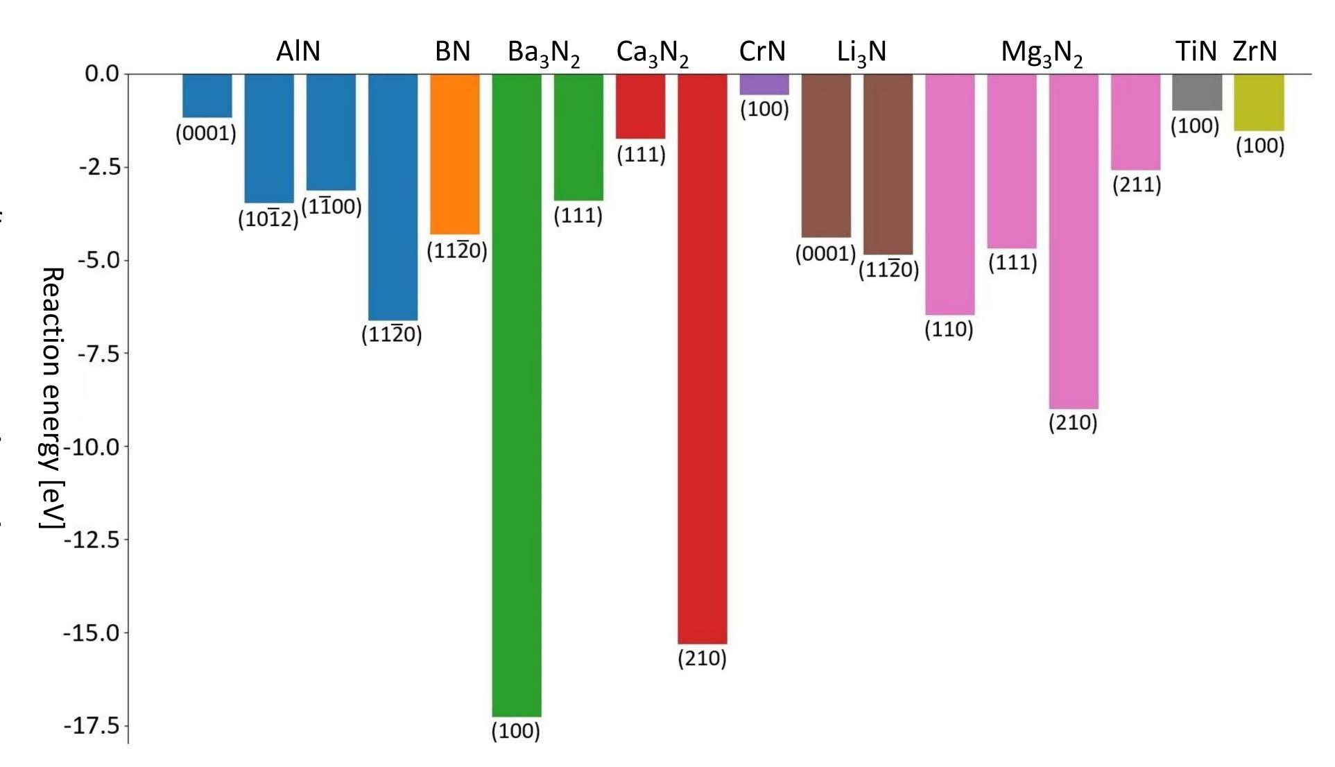
Reactions on all surfaces proceed with a negative reaction energy. Similar surfaces across the nitrides result in similar reaction energies. The reaction energies follow the trend that lower electronegativities of the metal centers (more ionic M-N bonds) result in more negative reaction energies.
