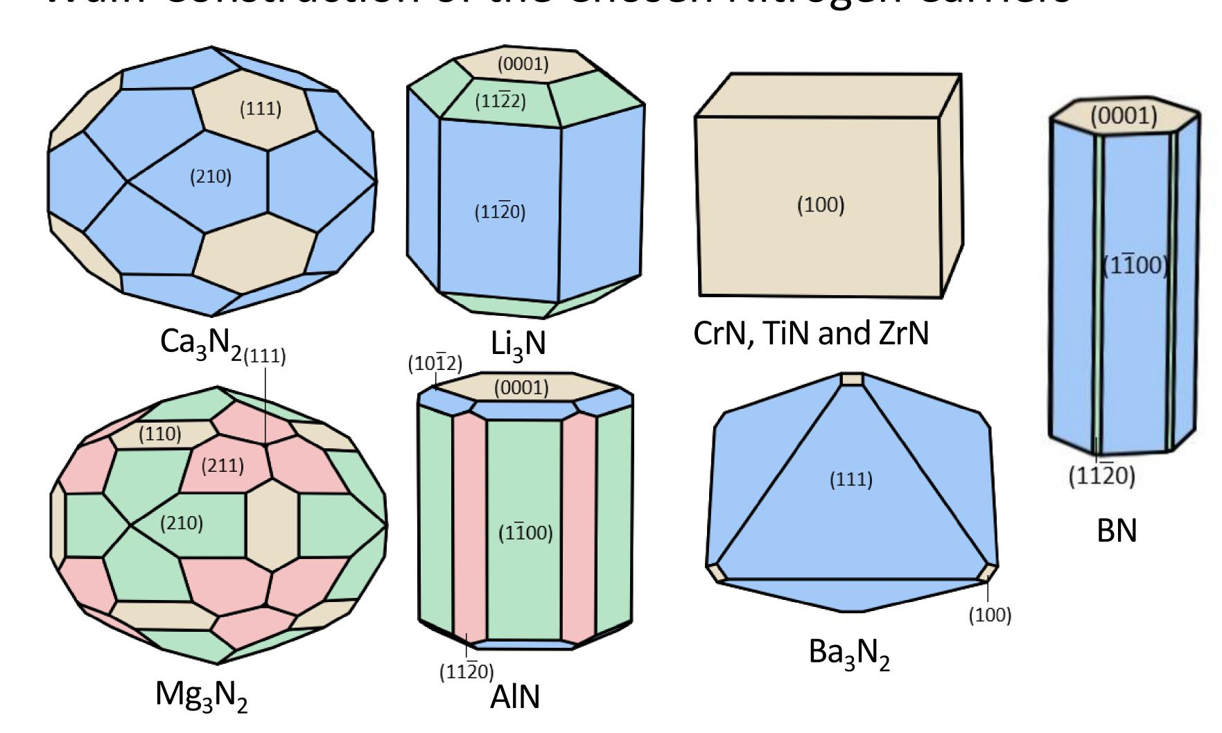
Only 1-4 different surfaces occur in the Wulff construction depending on the material. Same space groups exhibit similar surfaces (AlN and BN;  $Ba_3N_2$ ,  $Ca_3N_2$  and  $Mg_3N_2$ ). CrN, TiN and ZrN all show the same construction consisting of only the (100) surface.
