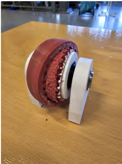
Figure 6.4: Critically damaged soft silicone roller
