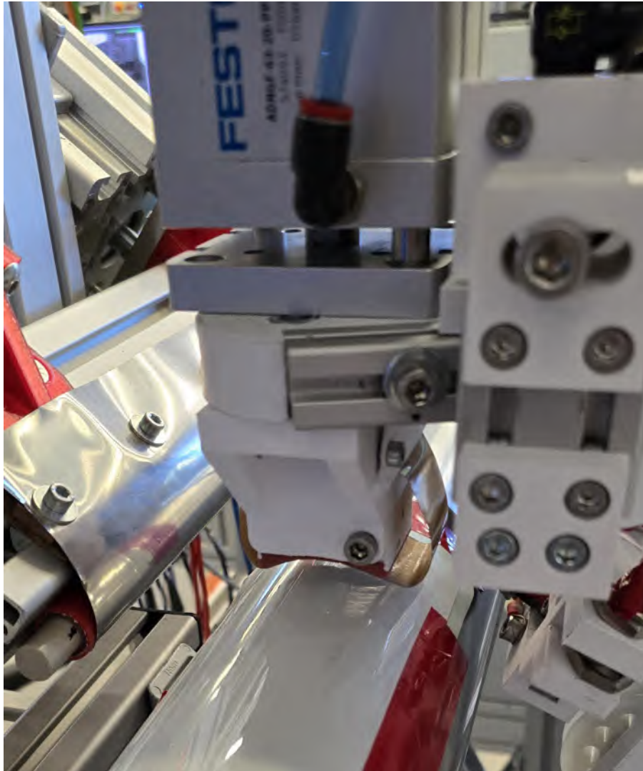
Figure 4.11: Setup for the static compaction trials, showing a slider lying above the Prescale films placed on the mandrel
