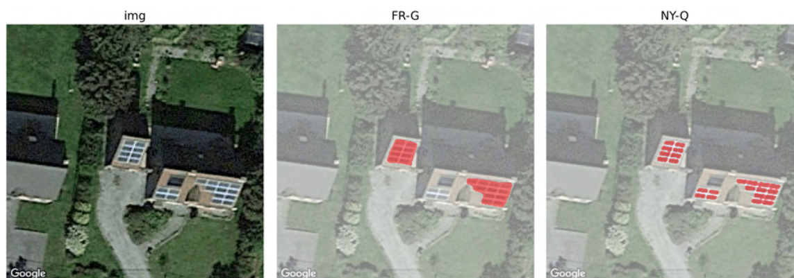
FIG. 1. Example of discretization of the individual array modules in an FR-G image when predicted by the NY-Q trained model.
