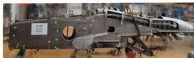
Fig. 5 Side view of a pylon of an A320 aircraft during a modal test
