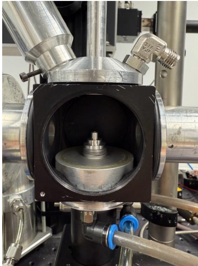
Figure 4.4: View inside the Process Chamber (Thorlabs cube)
