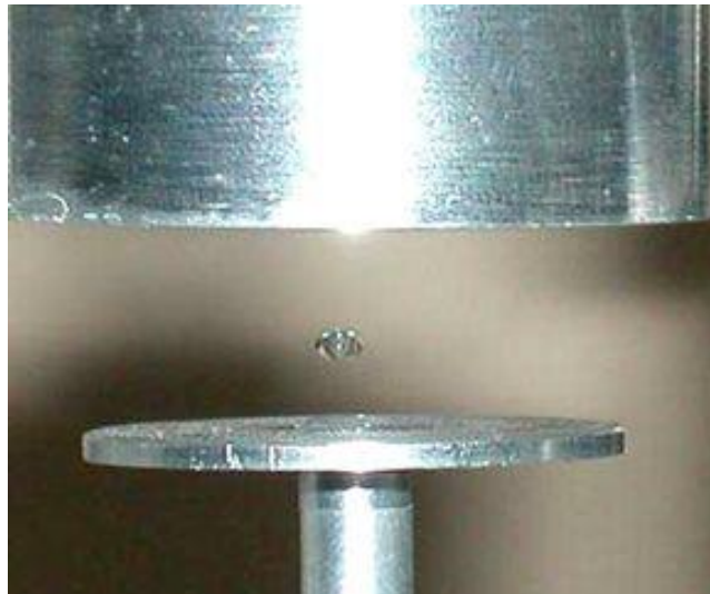
Figure 3.2: An experimental setup demonstrates acoustic levitation, in which a droplet is maintained in stable suspension at the node of a standing ultrasonic wave formed between a piezoelectric transducer located at the bottom and a reflector positioned at the top. [26]
