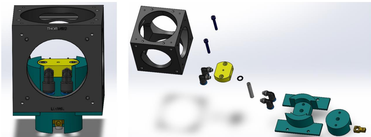
Figure 5.12: Assembly of the final reactor system including process chamber, nozzle unit, integrated water cooling, and embedded electrode. The right-hand side shows an exploded view of the reactor system
