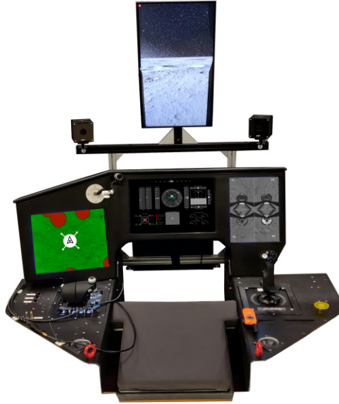
Fig. 26 Configured seating module for the Human-In-The-Loop (HITL) LL simulation. The top screen acts as a virtual window to the outside. Digital instruments are displayed over the three front screens. A force side-stick and a throttle lever are the main HMI's used to pilot the LL.
