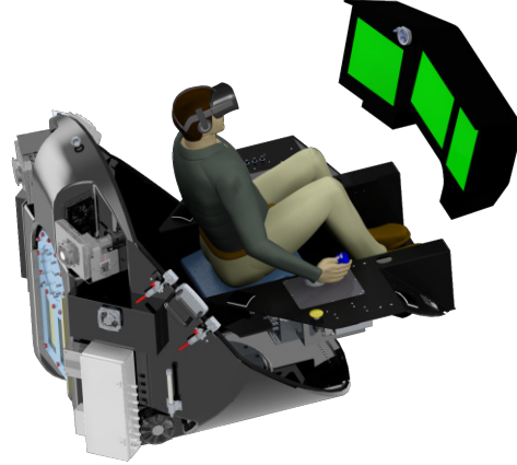
Fig. 24 Exploded view of DLR RMS's simulator cell showing its modular design.
