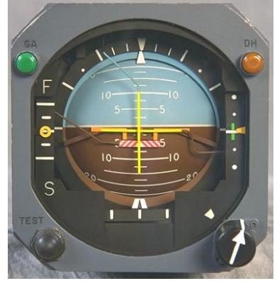
Fig. 16 An example of an artificial horizon gauge.
