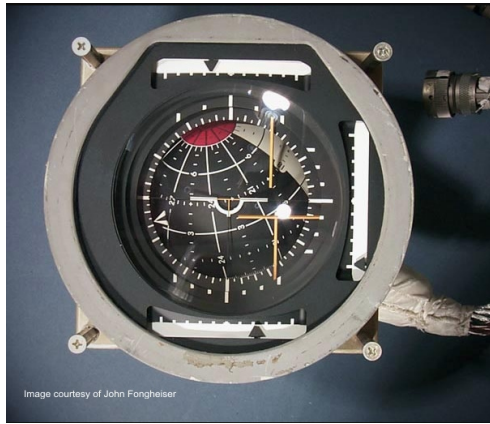
Fig. 2 NASA's Flight Director Attitude Indicator (FDAI)
