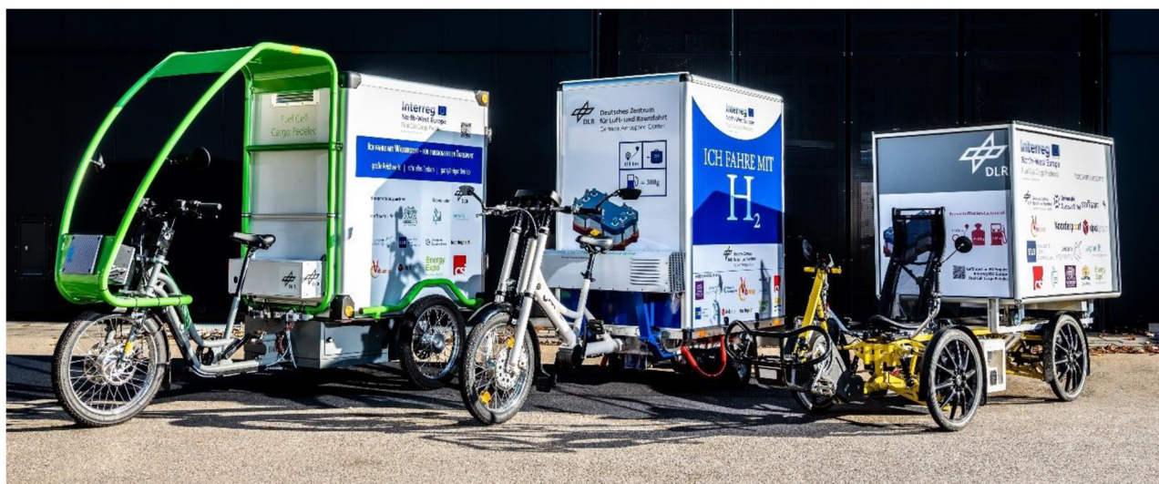
FIGURE 2 Three examples of the trialed fuel cell cargo pedelecs: Bring S by Bayk, UM CargoBike by Urban Mobility, Amadillo by Velove (photo: DLR).
