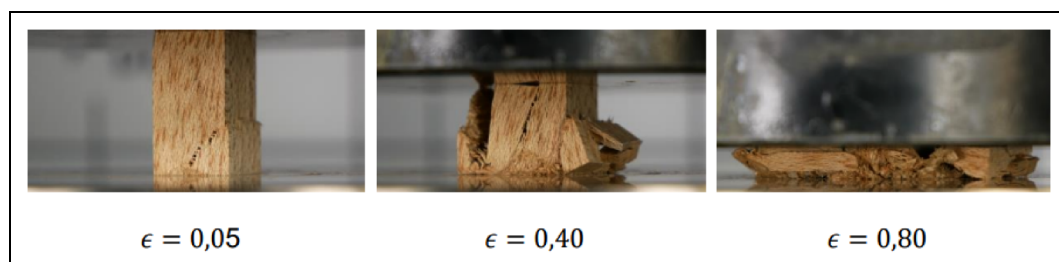
Figure 3. Compression tests of Albasia solid wood parallel to the grain at different strains 17 showing the fracturing of the material.
