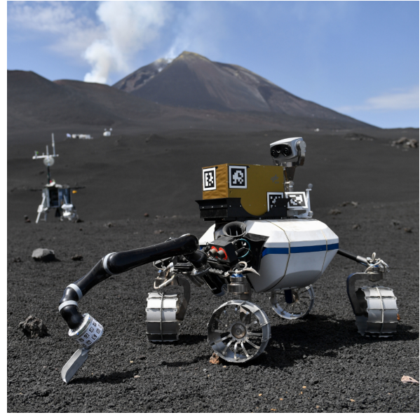
b) LRU2 shoveling soil. ©DLR/Oprean
