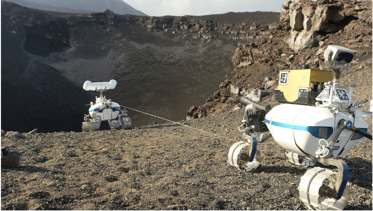
Figure A.2 Cooperative exploration of the Cisternazza crater in the context of the ARCHES space analog mission in 2022 on Mt. Etna. LRU1 has the winch mechanism mounted on its body. The end of the tether is connected to a hook, which is clutched to the robot arm on LRU2. From [Bur+24].
