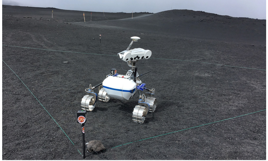
Figure 4.3 The LRU1 at the calibration site on Mt. Etna. A static reference coordinate system is created manually at a sloped, approximately planar test area.
