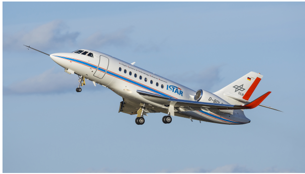
Fig. 1. The DLR ISTAR research aircraft with installed nose boom. Source: Uwe Bethke, Braunschweig.
