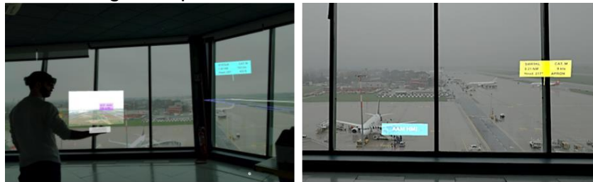
Figure 3: Integration of XR-based HMIs in the Bologna Airport scenario: Real-world implementation combining simulated ground infrastructure and unmanned traffic with a real-time AR interface for airport traffic monitoring, as viewed through a Microsoft HoloLens2.
