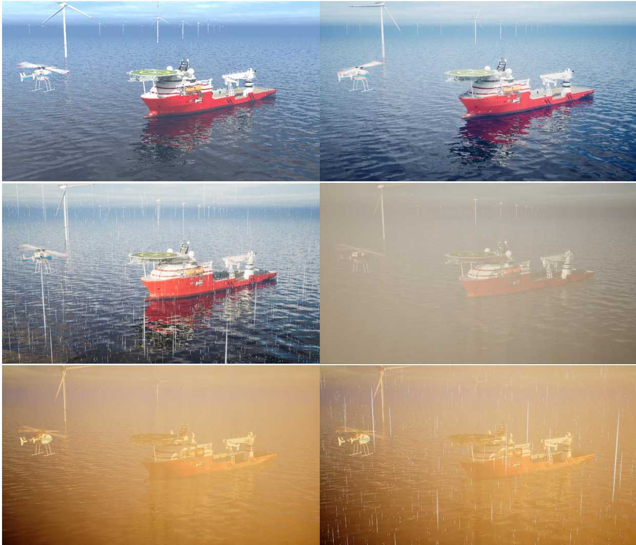
Figure 3, a-f: Simulation of different ODD parameters utilizing the SenSim2 framework, showcasing effects of rain, snow, fog, and daylight.
