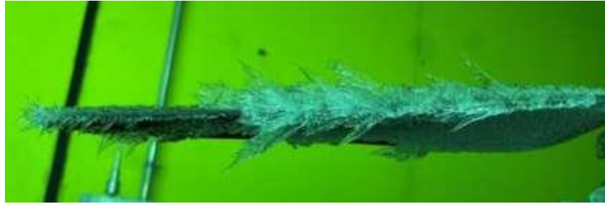
Figure 2: Severe ice accretion on a multi-copter propeller
