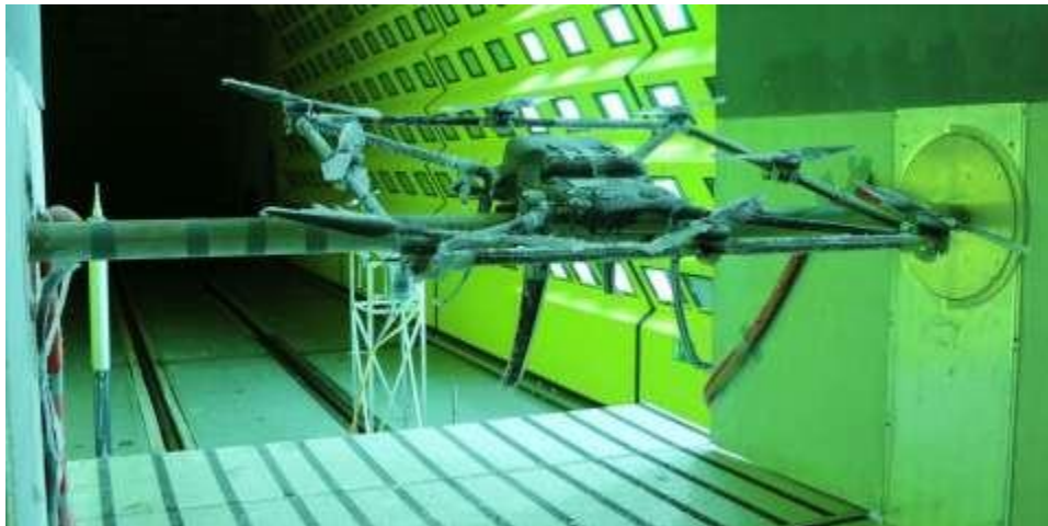
Figure 1: The 25 kg multi-copter UAV in the climatic wind tunnel.
