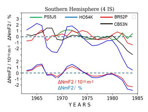
Linear models of NmF2 by the F30 solar radio flux indicate only small errors at all ionosonde stations in the order of about 1-2 %.
