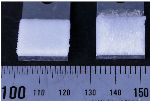
Fig. 12 Rime ice generated with the icing wind tunnel (left) and the ice printer (right).
