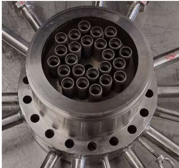
Figure 2 : Additively manufactured swirl-injector head
