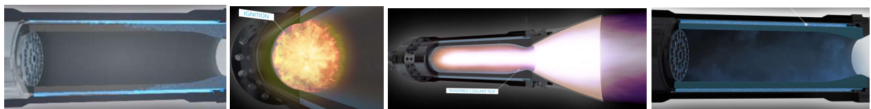
Figure 4 : Wall transpiration is activated before ignition (a), during ignition (b), during steady-state operation (c) and after extinction (d)
