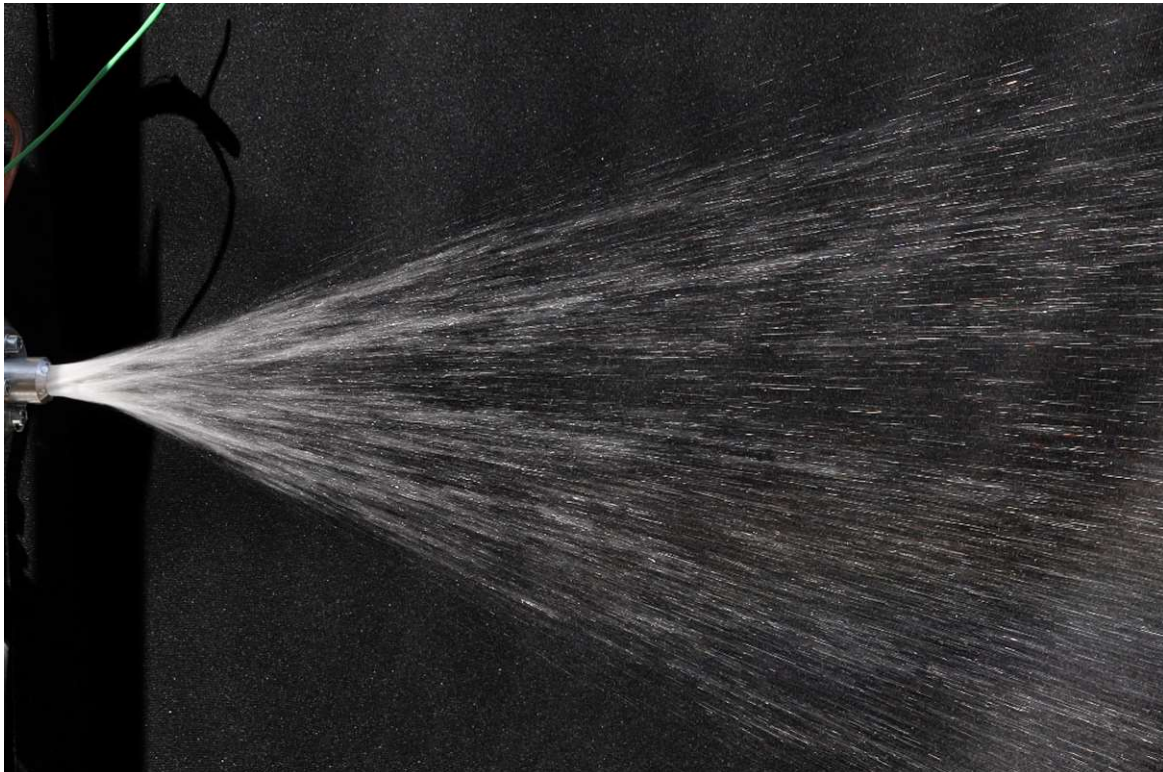
Figure 11: Pure water flow through LOx channels with increased speed at relevant mass-flow level for LOx simulation.
