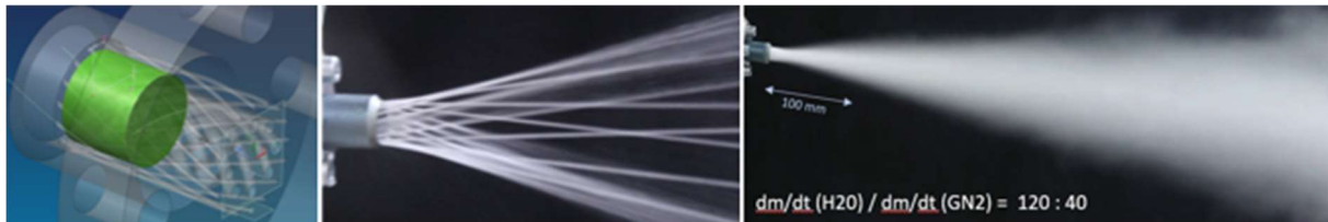
Figure 1 : CAD of the swirl channel design (left), resulting spray pattern using water (middle) and spray behavior (right)
