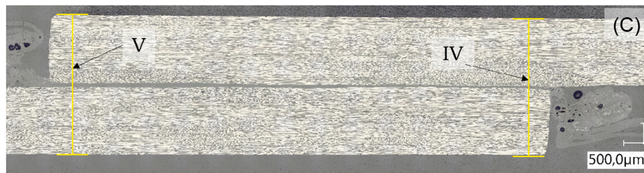
Fig. 16. Micrograph image of material #03, power-controller, weld number #05, section position #03, evaluation example (C) showcasing the displacement measurement position (IV) and (V).
