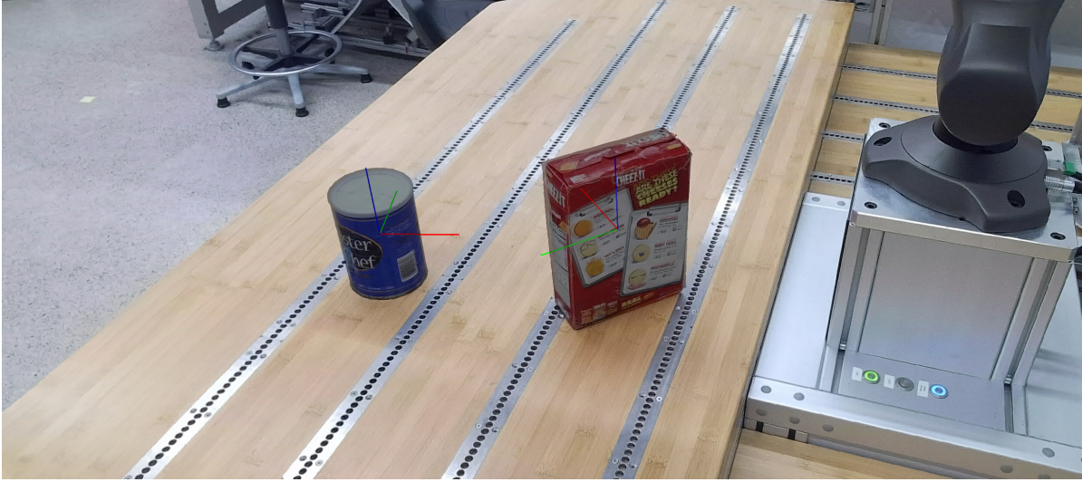
Figure 4.3.: Example output of the object pose estimation pipeline. The estimated 6D poses of detected objects are visualized by overlaying their coordinate frames on the captured image. The red, green, and blue axes represent the x-, y-, and z-axes of each object frame, respectively.
