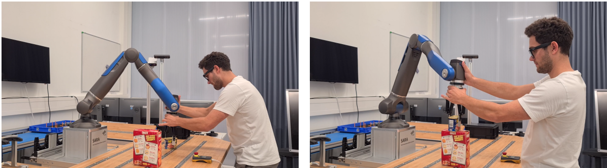
Figure B.1.: Images used to generate the schema for the skill SkillStackObjects (see subsection 4.1.2). The images were manually selected, since the perception module is not part of the framework (see subsection 4.1.1). (left) Grasping stage. (right) Stacking stage.
