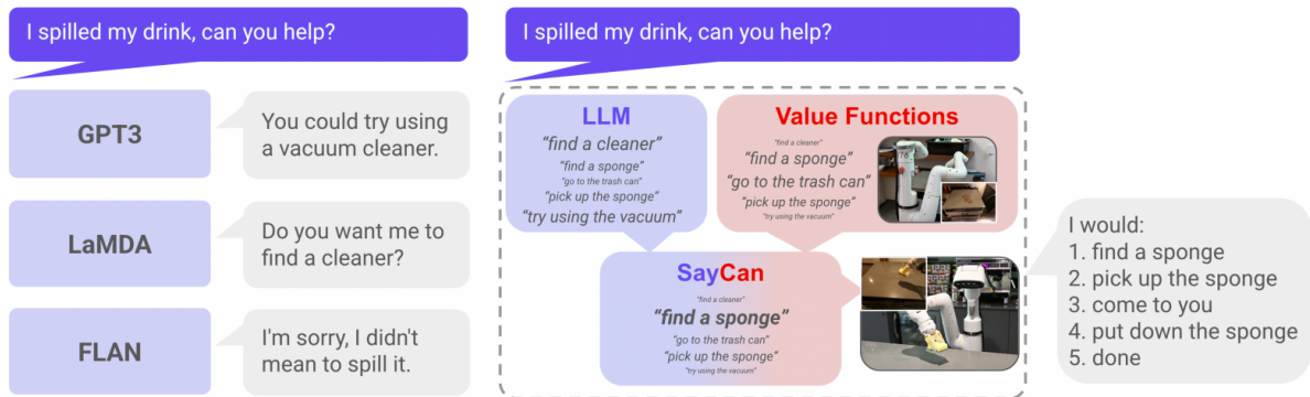
Figure 2.2.: Overview of the SayCan framework [61]. The system combines LLM probabilities for task usefulness with value function probabilities for execution feasibility to select skills that are both semantically appropriate and physically achievable. Image credit: Ahn et al. [61].
