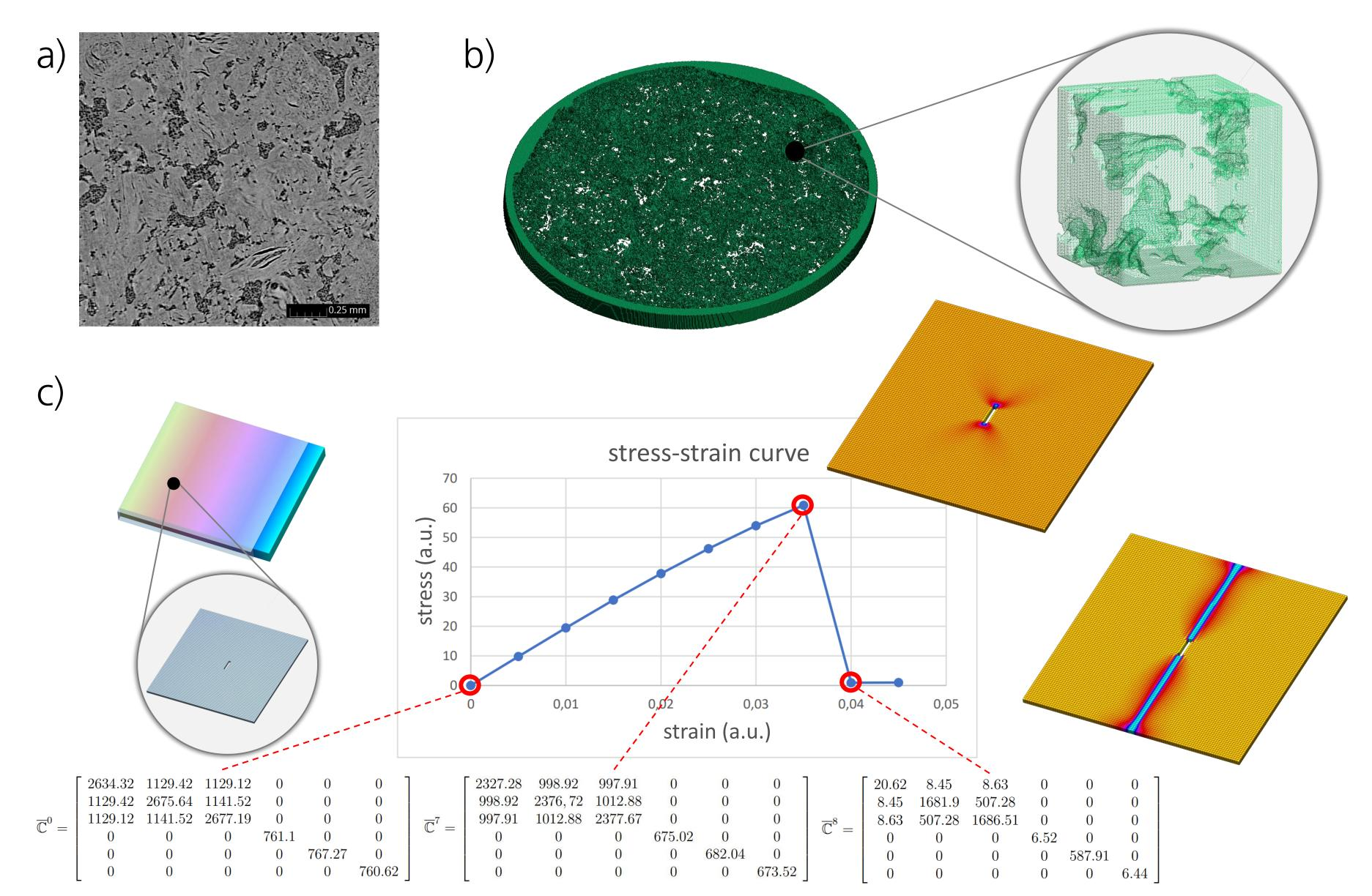
a) Slice of a CT scan of Diabon, light areas are graphite, dark areas are phenolic resin b) Digitalised microstructure of Diabon showing graphite and resin volumes c) Progress of a coupled FEM simulation for crack propagation using a phasefield model in an anisotropic artificial material and homogenised tensors of elastic constants of the entire plate
