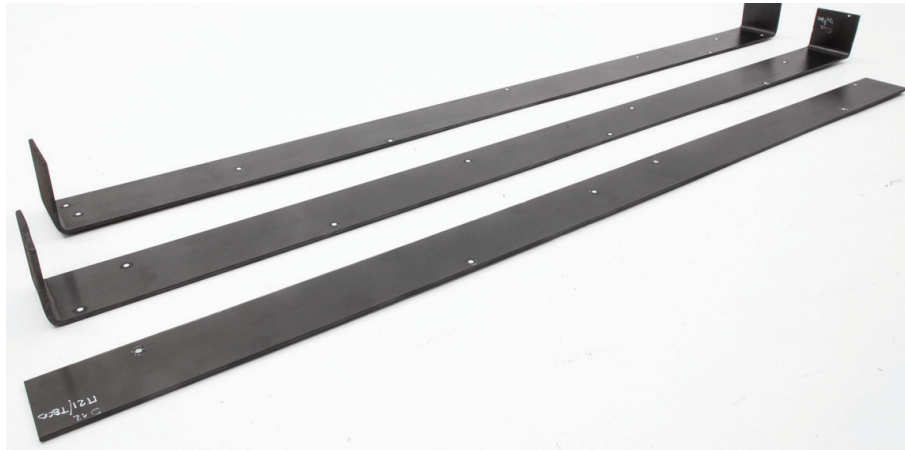
Fig. 5.17: Fabricates specimens to characterize the forced-interaction effect. C-shaped and I-shaped parts have a web-length of 798 mm and 754 mm respectively.
