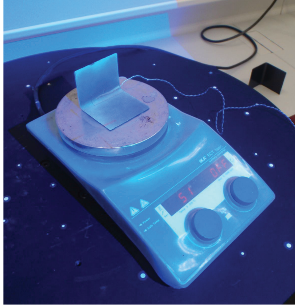
Fig. 4.42: Specimens applied on the hot-plate during the measurement
