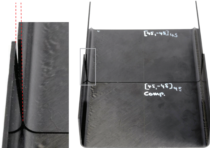
Fig. 7.8: Effect of the tool compensation. Distance between red lines is approximately 2 mm
