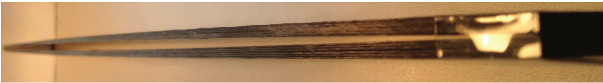
Fig. 5.15: Flange warpage of the separated flanges is obtained to 2.385 mm. Flange centers warp away from the tool
