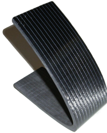
Fig. 7.16: Small demonstrator of a CFRP leading edge as an example of a curvature changing structure. Picture taken from [100]
