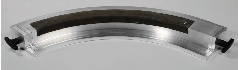
Fig. 4.47: Aluminum tool for curved L-profile specimens
