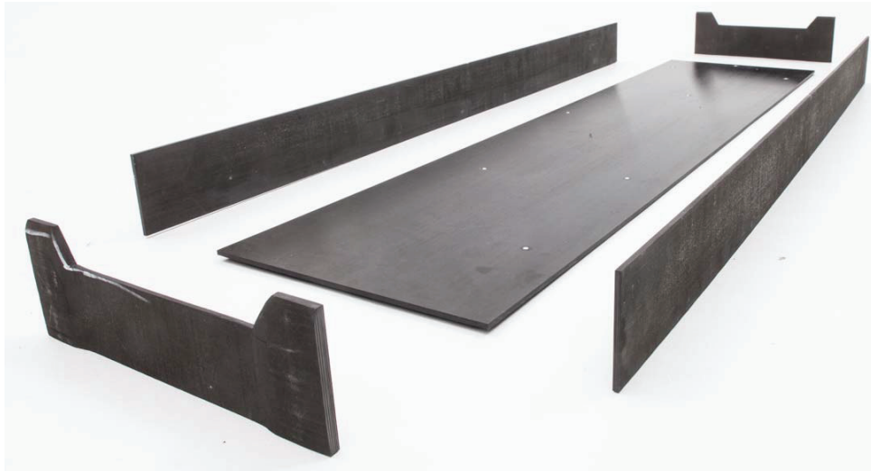
Fig. 5.13: Box specimen after separating with a diamond saw
